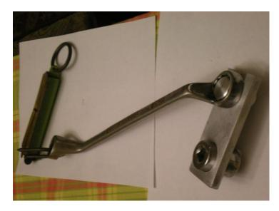
Tool shown with socket and adapter in place and with ring spanner and fish scale used to apply torque
